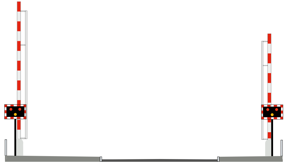
Standard wigwag lighting and barriers
