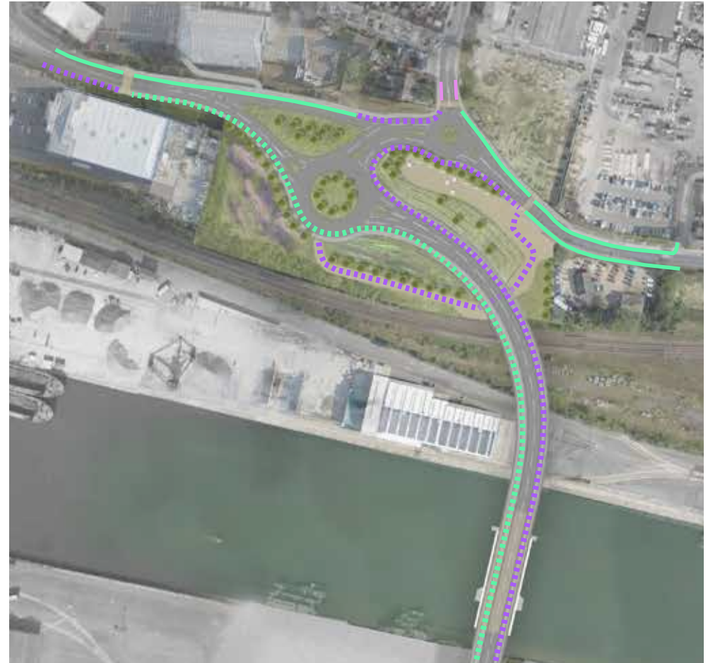
Reference design - Northern approach: Cycle facilities
