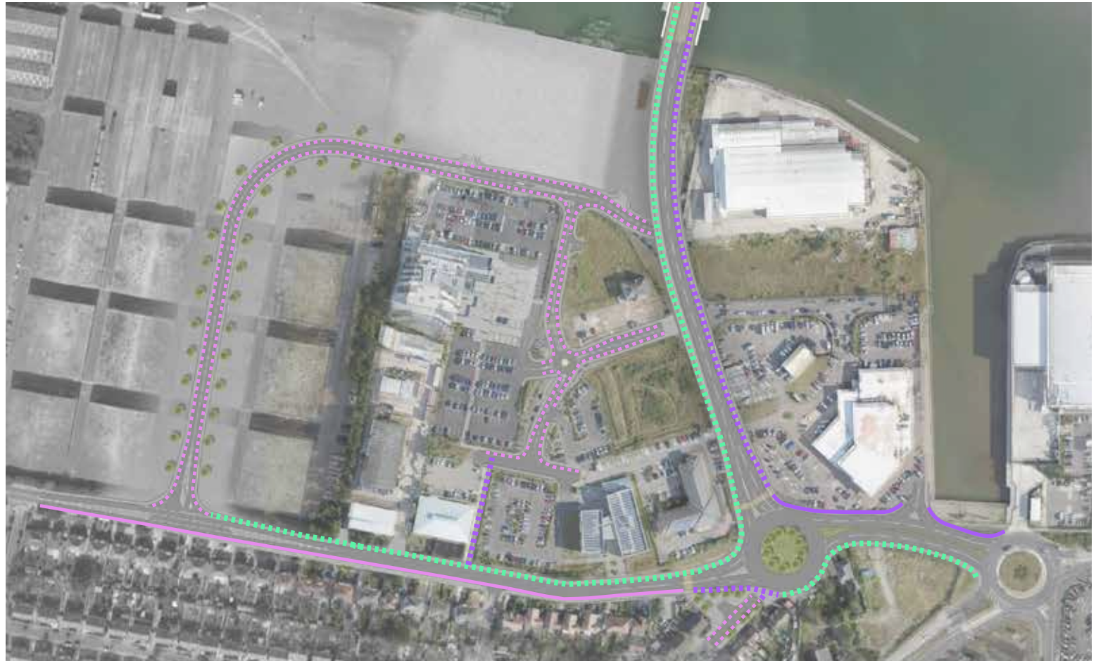
Reference design - Southern approach: Cycle facilities
